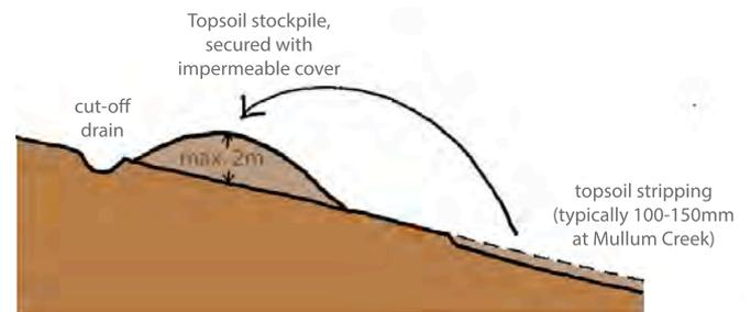
Figure 5: Topsoil stockpiles.
