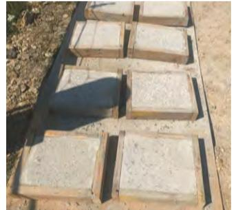
Figure 8: Excess wet-mix concrete pavers
